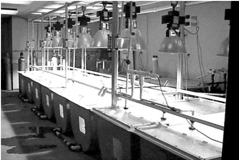
Fig. 1. The experimental HISTAR system contains two enclosed turbidostats (foreground) and six open-topped continuous-flow, stirred-tank reactors (CFSTRs, background).
