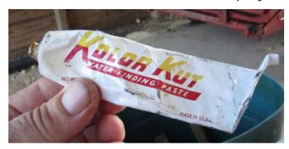
Kolor Kut (or equivalent) paste can be added to the end of a rod or wooden dowel and submerged into the bottom of the fuel tank to test for water contaminated diesel fuel. If it changes color then your fuel is contaminated with water, the culprit behind many fuel problems.
