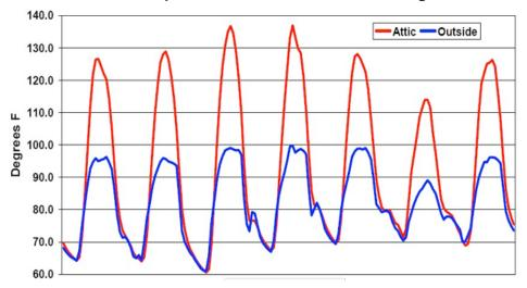
Outside vs attic data in summer for the same house shows attic temperatures typically not rising above outside temperatures until outside temperatures are near or above 90 F. Little to no benefit from attic air inlets can be expected in this situation.
