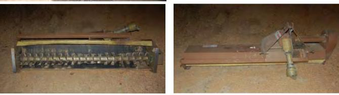
A shallow-tine roto-tiller is an excellent tool for conditioning litter after decaking. Growers should be aware that tilling too deep can contribute to ammonia problems. This shallow tine tiller, which can be pulled behind a 40 hp tractor and do a typical house in less than an hour, is often used to depths of only 1 to 2 inches to mix and condition the surface after decaking.
