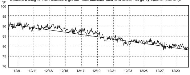
**Datalogger shows temperature variations during first 21 days of broiler growout** – Grower can look at a chart of this type to check how closely in-house temperature is being held to target, and make equipment, management and/or controller adjustments needed. This record shows a good environmental control job, with few temperature swings of more than a few degrees above or below optimum target.
