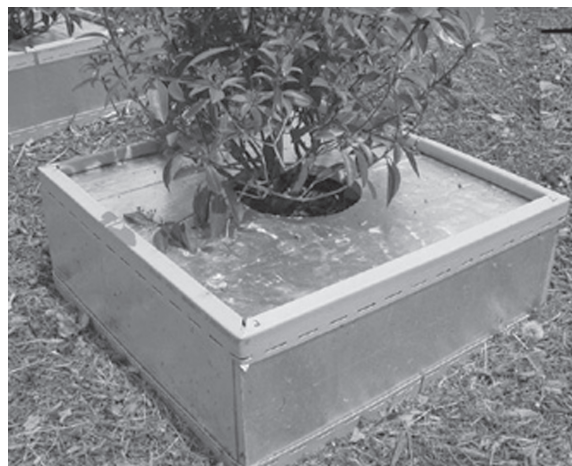
Fig. 4. Exterior walls of Horhizotrons assembled outdoors were placed directly on the ground. The upper lid shown has portions cut out to expose the substrate surface immediately around the plant stem (same lid as for Horhizotrons used indoors).
