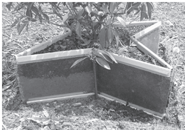
Fig. 3. Horhizotrons were constructed for outdoor use by assembling quadrants directly on the ground and eliminating the aluminum base and wood frame.
