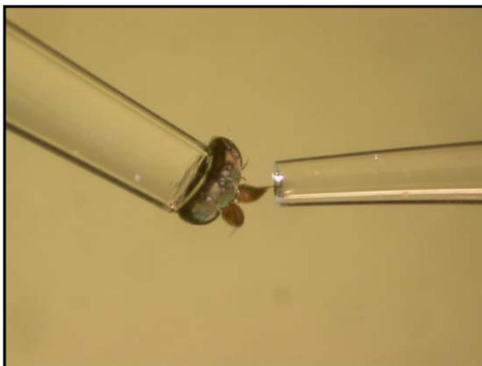
**Figure 3:** Preparation for studying electroantennogram (EAG) response of phorid flies to fire ant odor (the head of phorid fly placed in between two glass electrodes).
