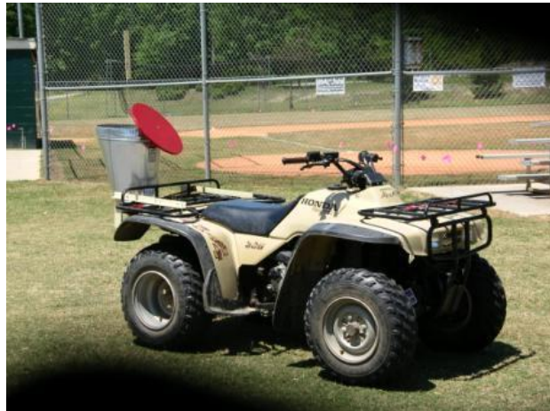
ATV with Herd Seeder attached for fire ant bait application.
