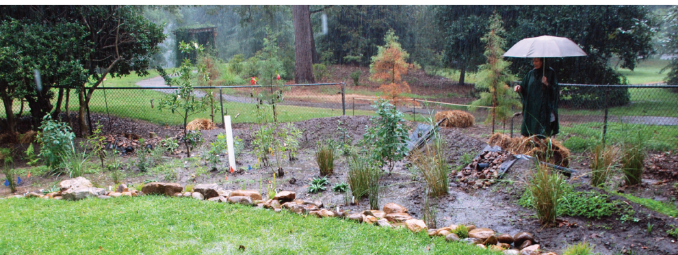
EASING THE FLOW Arboretum curator Dee Smith points out a rain garden that was installed at the facility to manage stormwater runoff by catching rainwater where it falls.
