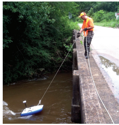
FLOOD PREVENTION Associate professor Latif Kalin uses a hydroacoustic current meter to measure how fast and deep the water in Eightmile Creek in Prichard is during a flood event. Kalin and colleagues have developed a method for identifying sensitive areas in a watershed that, if they were to be developed, could contribute to downstream flooding.
