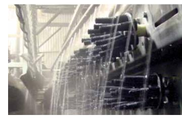
FLOWING FREELY—Water sprays from nozzles on a featherpicking machine at a poultry processing plant even though the processing line is idle. This plant has six pickers with a total of 252 nozzles. The Auburn water-use auditors concluded that leaving water running at the pickers unnecessarily wastes 18,182 gallons of water daily and 4.7 million gallons—and \$8,299—annually.
