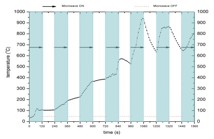
Temperature profile of bulk corn stover during microwave-induced pyrolysis
