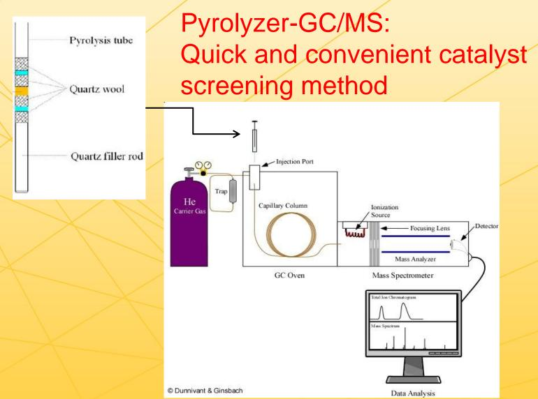
Biomass (yellow) is pyrolyzed in the quartz tube and vapors go through the catalysts bed (blue) and then analyzed by GC/MS. UNIVERSITY OF MINNESOTA
