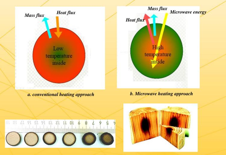
c. Pyrolysis front development with conventional heating d. Pyrolysis front development with microwave heating
