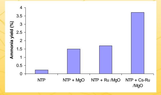
NTP Ammonia synthesis different catalysts.  $(V_{N2}:V_{H2}=1:3, N_2 \text{ and } H_2 \text{ total flow rate 60ml/min, voltage 5000V, frequency 8000Hz.})$
