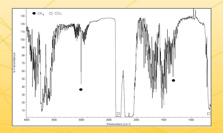
FT-IR spectroscopy of NTP reforming of CO and H<sub>2</sub>O vapor.
