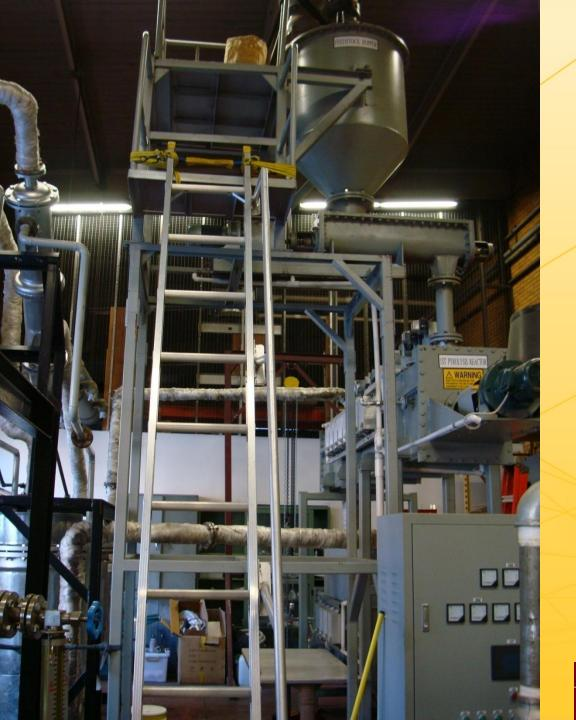
Continuous microwave assisted pyrolysis system development
