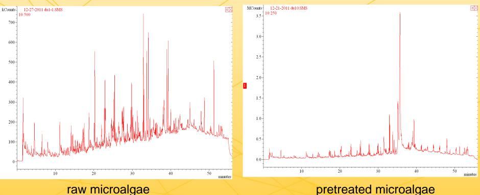
The pyrolytic bio-oil from pretreated algae contained less Ncontaining compounds and the bio-oil contained mainly long-chain fatty acids (C14–C18, over 45%) which can be more readily converted into hydrocarbon fuels in the presence of simple catalysts.
