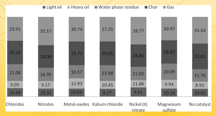
Pyrolysis fraction yields (mass% of total biomass input) from runs with different catalysts and catalyst groups added to the **aspen** pellets
