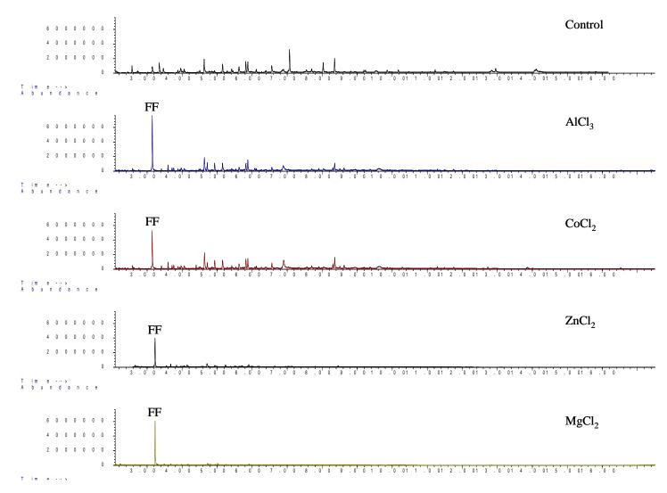
Total ion chromatograms from GC-MS analysis of pyrolytic oils from corn stover when different catalysts were used (8g/100g biomass). FF: furfural.
