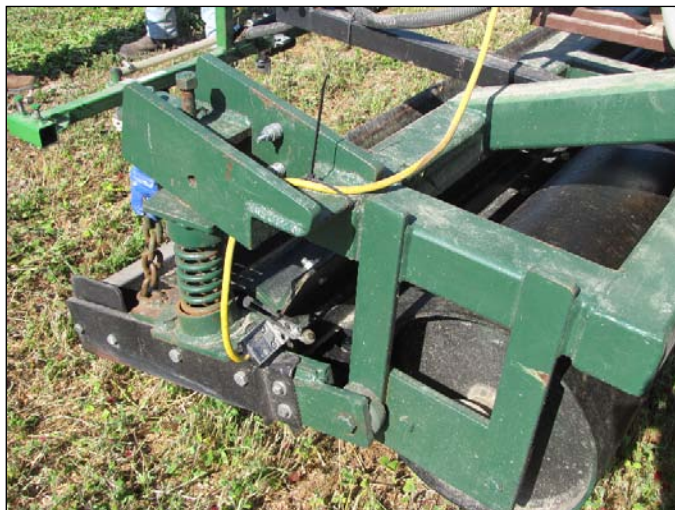
Figure 3. Two-stage roller/crimper with the electric switch mounted on the pivoted roller's frame to be energized by the 1/2 inch DIA engagement bars mounted on the crimping bars of the crimping drum.
