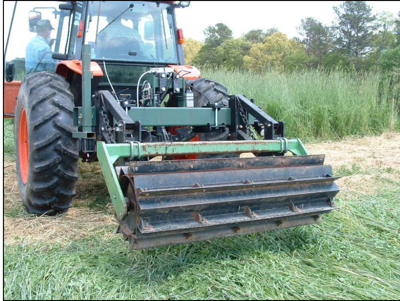
Figure 1. Rolling cover crops using a 8 ft straight bar roller/crimper with \frac{1}{4} inch thick crimping bars
