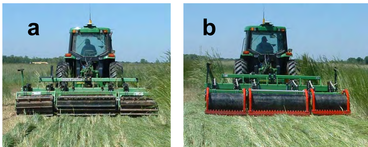
Figure 1. Three-section roller types: (a) Straight bar roller, and (b) Smooth roller/crimper.
