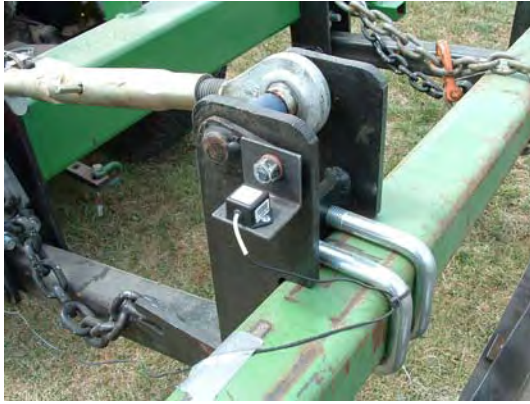
Figure 2-Location of accelerometers mounted: (a) roller's frame, (b) Tractor's frame
