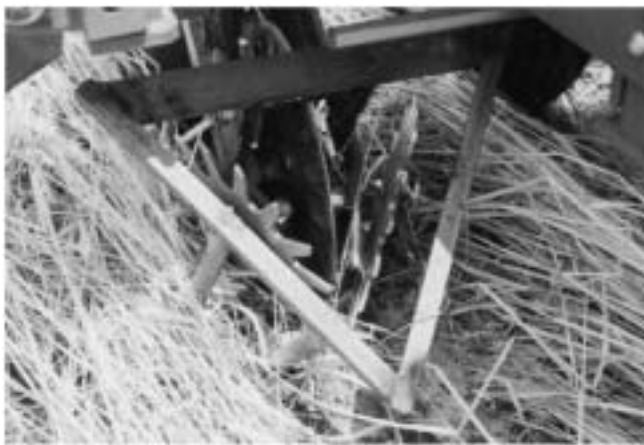
Fig. 4. Cotton planter with a forward residue mover.
