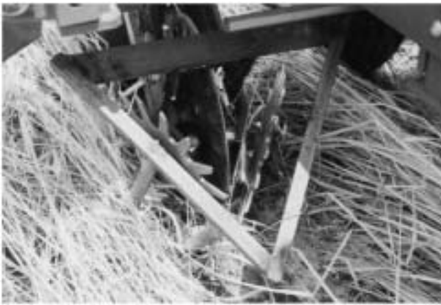
Fig. 4. Cotton planter with a forward residue mover.
