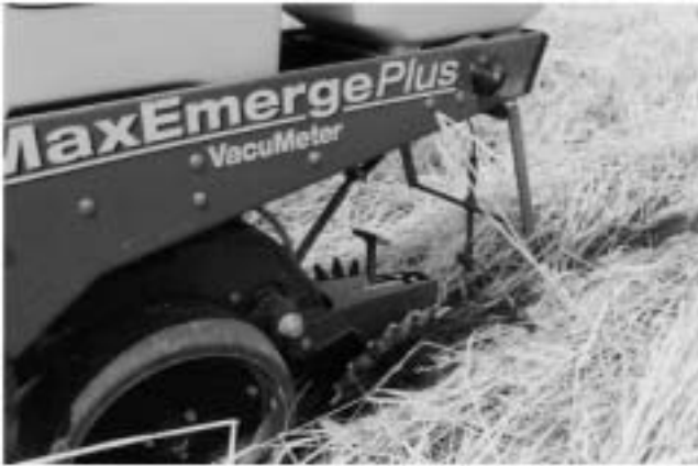
Fig. 3. Cotton planter with spoked wheel row closers.
