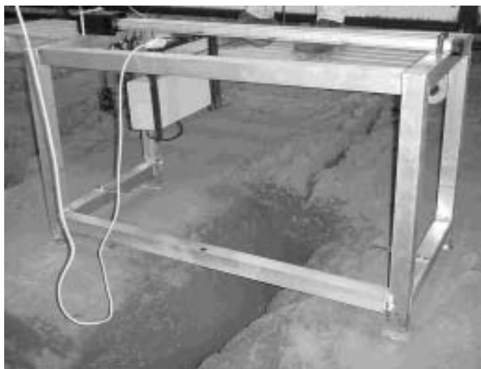
Fig. 2. Laser profilometer used to measure area of spoil and trench.
