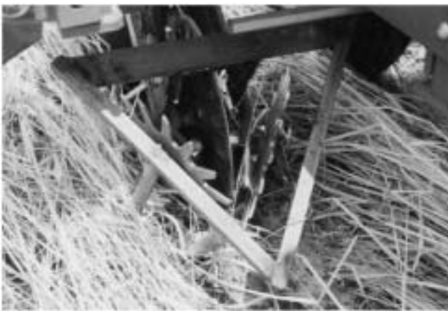
Fig. 4. Cotton planter with a forward residue mover.
