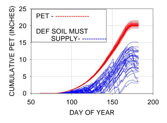
Fig. 1. Assessment of annual portion of evaporation that must be supplied by stored soil water to meet evapotranspiration demands, where PET refers to potential evaporation transpiration and DEF refers to moisture deficit that must be supplied by soil to meet PET.
