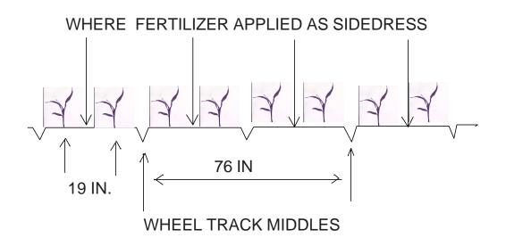
Fig. 3. Proposed seedbed preparation and planting pattern plan to alleviate surface drainage, soil compaction, and fertilizer burn problems.
