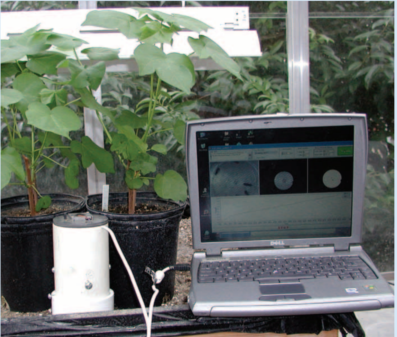
The Wasp Hound is connected to a laptop computer with live video of wasps shown on screen.
