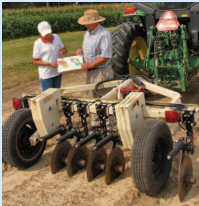
The VERIS 3100 instrument was used to create soil electrical conductivity maps. The instrument can be pulled behind a tractor or truck at speeds of up to 15 mph.
