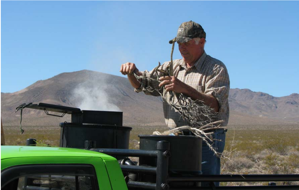
Wayne putting some desert scrub into the gasifier before getting to Death Valley
