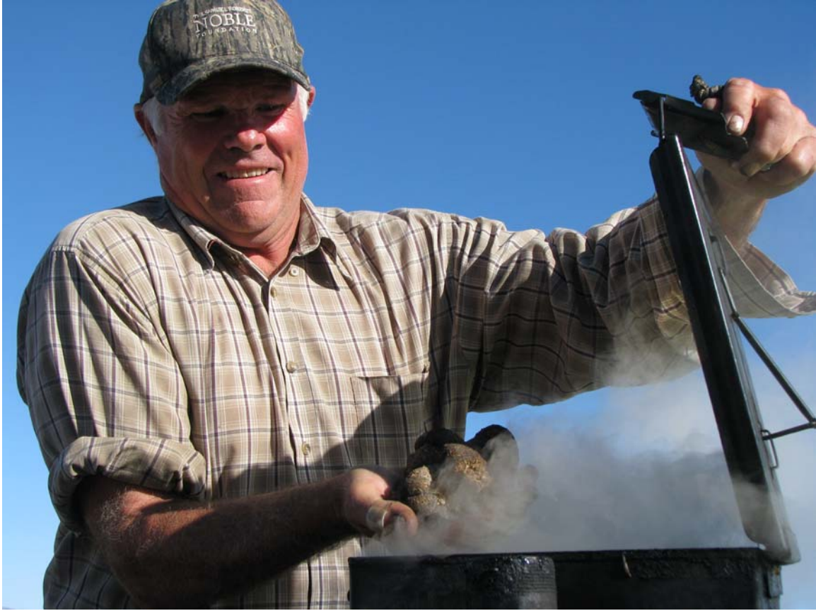
Wayne putting the horse manure into the gasifier
