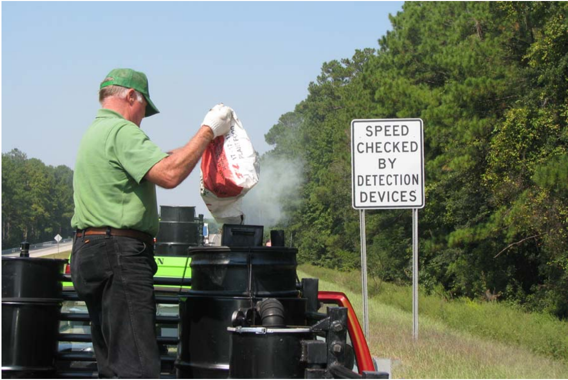
Filling up with wood on I-16 en route to Soperton, GA.
